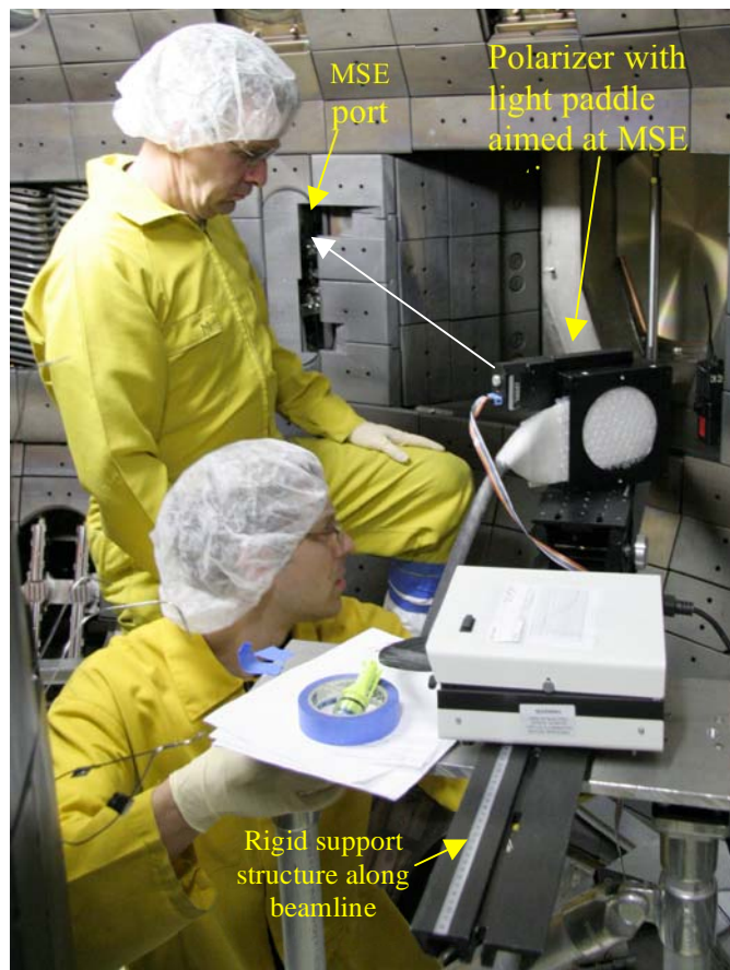
Figure 1. Basic MSE calibration on DIII-D.
