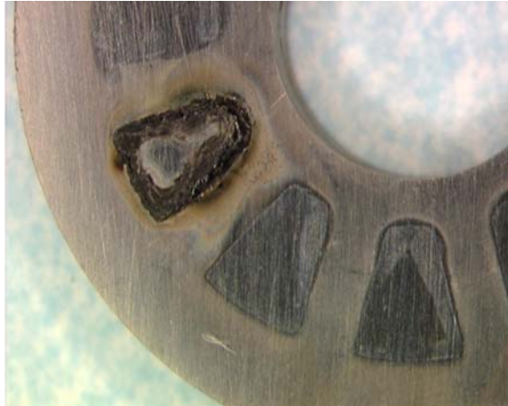
Figure 9. Specimen ASW MCA JE0138. One spot of major crevice corrosion and general corrosion in non-crevice areas. Magnification X8.
