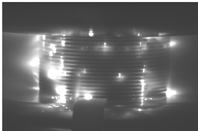
Fig. 11. HGI "R011." Thick-metal HGI undergoing representative surface flashover event. Sample height is 12.36 mm.
