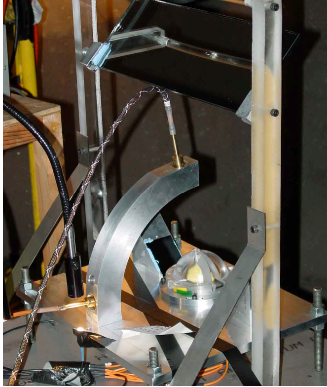
Fig. 2 Mirror and probe configuration for the scaling experiments.
