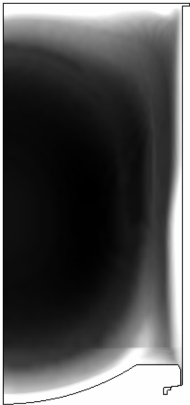
Figure 8. CO distribution for the phi=0.08 case @ EVO. Dark=high, light=low concentration.
