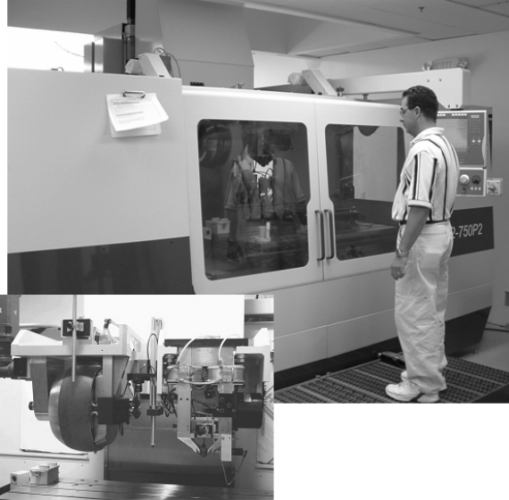
Figure 5: Large-aperture MRF designed and built to final figure and imprint CPPs uses two wheels, one large and one small, to imprint topographical features down to spatial periods of 1 mm. The MRF is capable of polishing optics up to 750 X 1000 mm in size.
