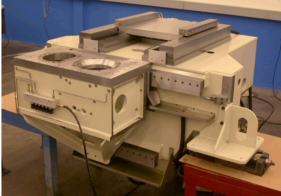
Figure 8. POGAL base and slides during construction at Moore Special Tool Company.
