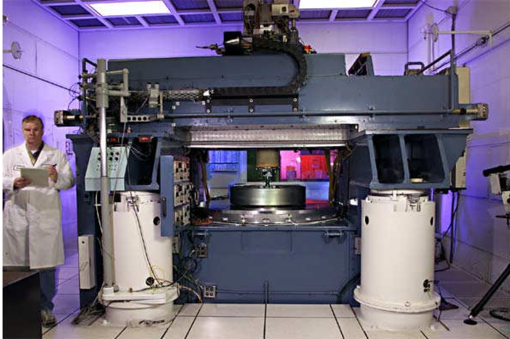
Figure 3. This is the Large Optics Diamond Turning Machine (LODTM) in its environmentally controlled room. The large work volume at the center is clearly visible.
