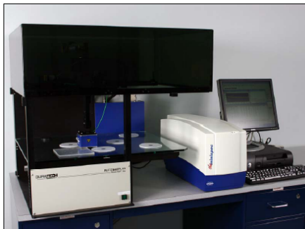
Figure 6. Robotic Autosampler designed by Bruker and DuraTech. A similar autosampler will be installed at KCP.
