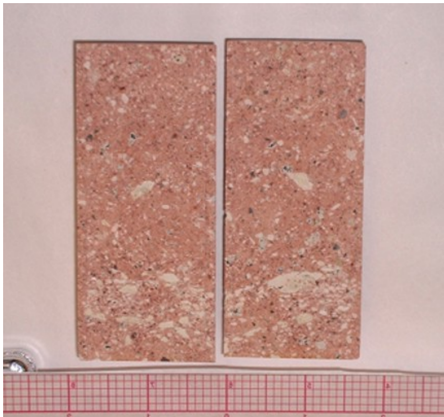
Figure 8.4. TCU-5 Synthetic parallel plate "slotted" fracture
