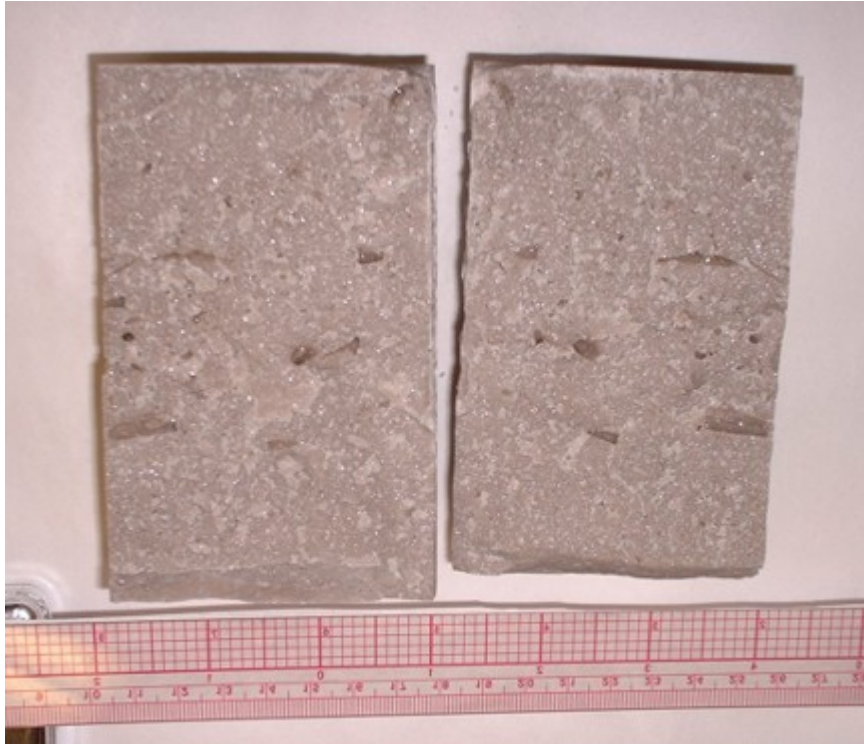
Figure 8.7. LCA-3 Brazil test induced fracture
