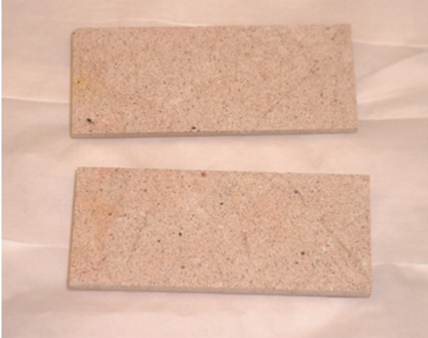
Figure 8.1. TCU-2 Synthetic parallel plate “slotted” fracture
