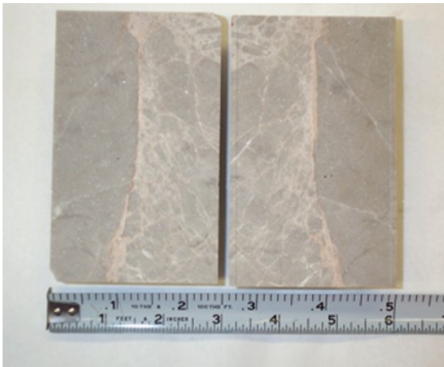
Figure 8.6. LCA-2 Synthetic parallel plate “slotted” fracture
