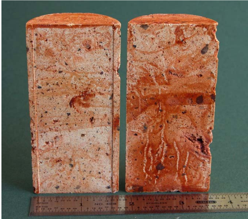
Figure 8.5. TCU-6 Iron oxide coated synthetic parallel plate “slotted” fracture
