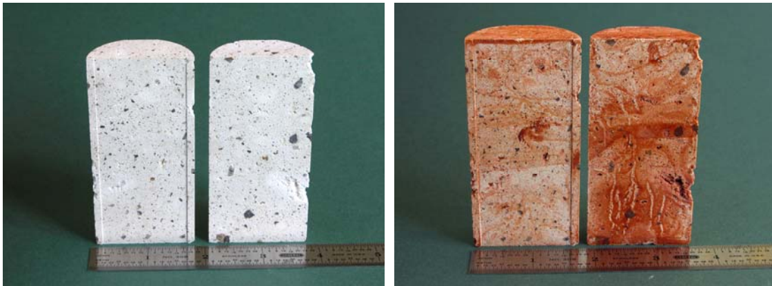
Figure 2.3. Photograph of natural tuff core UE-7az 1678.2-1679.0 on left, and same core on right after precipitation with iron oxide (TCU-6).
