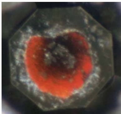
Figure 3. TATB pressurized to 16.4 GPa.
