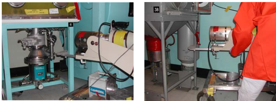
Figure 2. In-situ gamma spectroscopy of contaminated glove boxes and equipment
