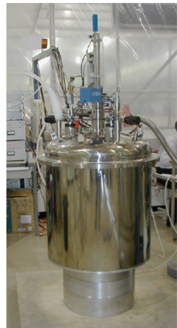
Figure 1 The Lujan Center's 11-Tesla superconducting magnet has an internal sample goniometer ( \pm 15^\circ about the neutron beam) and wide sample
