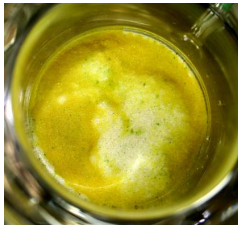
Photo 1: U crystal obtained in the crystallization tests with U-Pu-Cs solution (U: 409g/l, Pu(IV): 41.8g/l, Cs: 4.6g/l) (after washing). A small amount of whitish green crystals are observed in the yellow U crystal.
