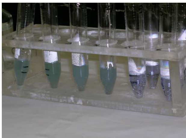
Photo A: After reduction to the Pu(III) oxidation state, the oxalic acid is added and the oxalate precipitate appears immediately.
