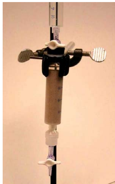
Fig 1: Experimental static column setup used for the investigation of the effects of EPS on plutonium sorption behavior.
