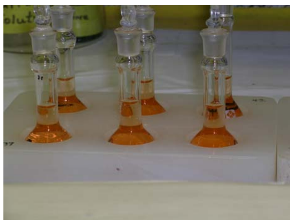
Photo B: After the reduction to Fe(II), the iron-orthophenanthroline complex forms.
