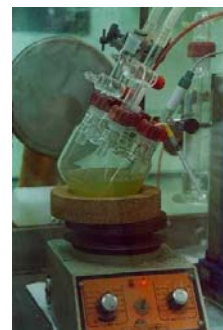
Fig 1: Reactor vessel used.
