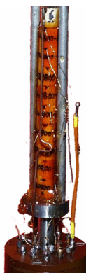
Figure 2. Sample holder and explosive sample. Burn wires are inserted through holes in Teflon® tube into sample. B/KNO_3 and HNS igniter and cardboard tube is on top, with igniter wires leading to it. Thermocouple in front is used to monitor temperature inside pressure vessel.
