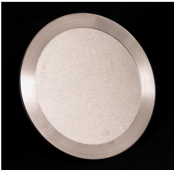
Figure 2. Photo of a zirconium/mesh spectral purity filter
