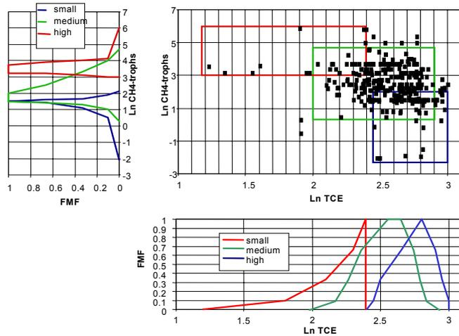
Figure 4. Fuzzy graph of the relationship between logarithms of TCE and methanotrophs concentrations for wells 1C-3C and 5C-10C and corresponding FFMFs plotted parallel to the axes.
