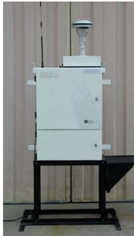
Fig. 1. One type of field aerosol collector used by the BioWatch system. Ambient air is drawn through the intake at the top of the unit, and passed through a filter to capture and retain any biological aerosol particles.
