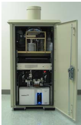
Fig. 2. The Autonomous Pathogen Detection System (APDS) is a self-contained biodetection system with automated sample collection, computer-controlled fluidics, wireless communications, and two independent types of bioassays.
