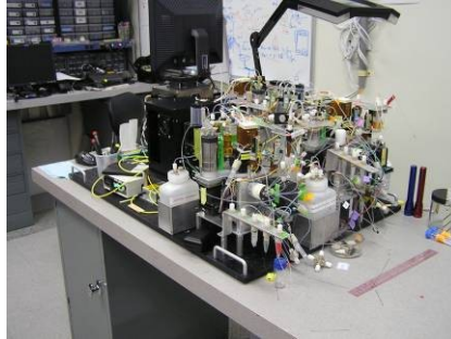
Fig. 3. A benchtop prototype of the BioBriefcase third-generation point detection system. Such systems contain miniaturized or microfluidic components, enhanced performance and extensive data networking capabilities.
