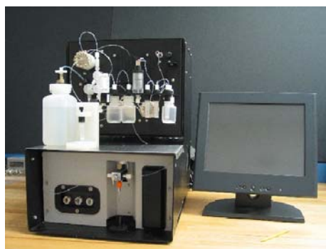
Fig. 5. The compact FluIDx unit is a point-of-care multiplex medical diagnostics system that uses the automated fluidics and bead-based immunoassay platform of the APDS. It has been used to rapidly diagnose viral upper respiratory infections.
