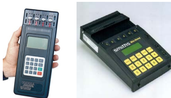
Fig. 4. The Handheld Advanced Nucleic Acid Analyzer (HANAA), at left, is an example of a field-portable biodetection system for use by first responders or decontamination crews. The core real-time PCR detection technology is also deployed in the commercial Bio-Seeq system (Smiths Detection), shown at right.
