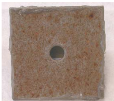
Type 316L Coating After Exposure for 13 Cycles
