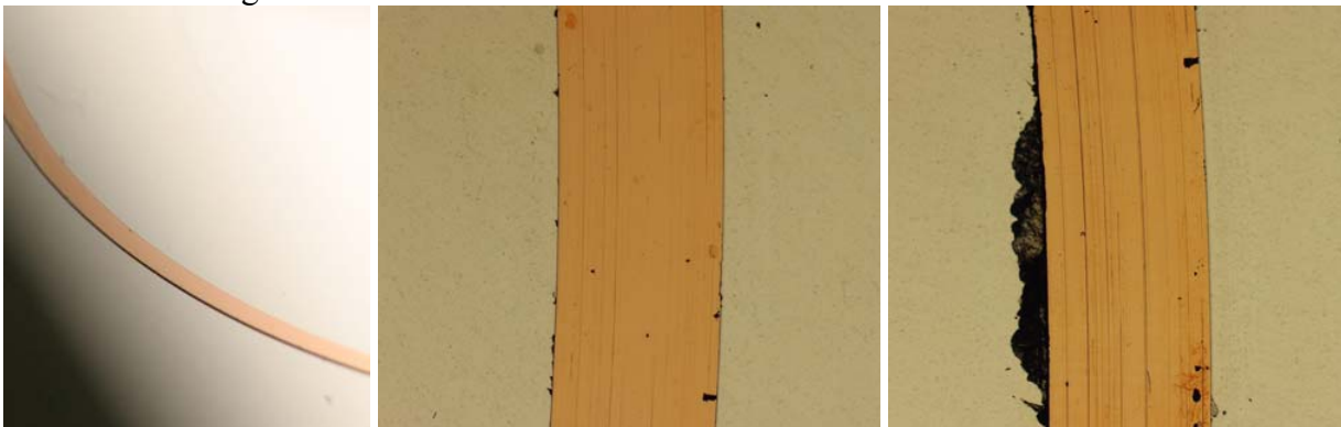
Figure 34. Disk SPUT11 after diamond turning the electroplated Cu
