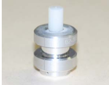
Figure 3. Standard Al holder used to mount workpieces on the DTM
