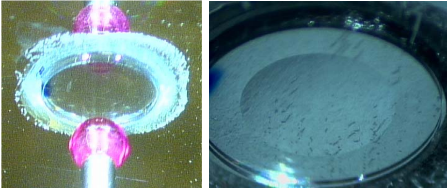
Figure 57. Chips sticking to the diamond turned UV curing adhesive and the ICH pad
