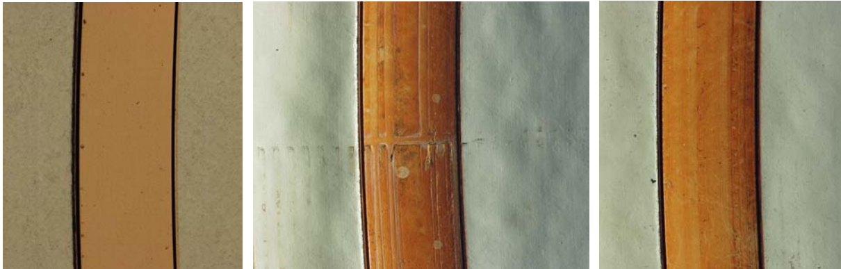
Figure 65. Freshly diamond turned 1 mm \times 43 \mu\text{m} band of Cu (left). Cu that was adjacent to the radial grooves in the vacuum chuck (center). Cu that was not adjacent to the radial grooves in the vacuum chuck (right).
