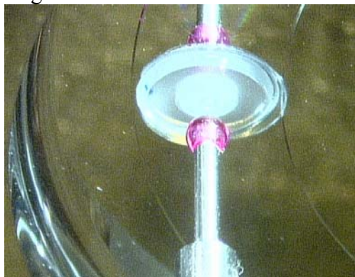
Figure 61. Measurement of adhesive layer thickness for an ICH pad
