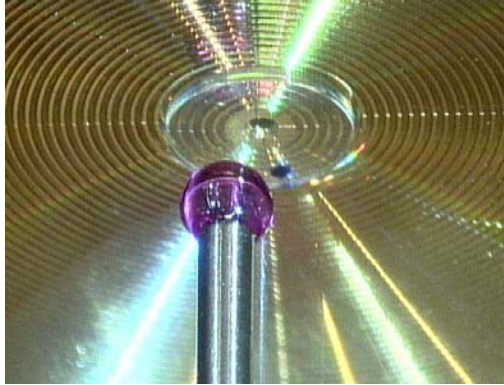
Figure 52. Measurement of thickness and thickness uniformity of a CH pad
