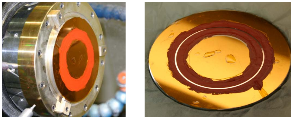
Figure 27. Disk SPUT3 after coating the Al and Cu with electroplating paint (left) and after scoring and peeling up the 1 mm wide section of paint that had covered the sputtered Cu (right)
