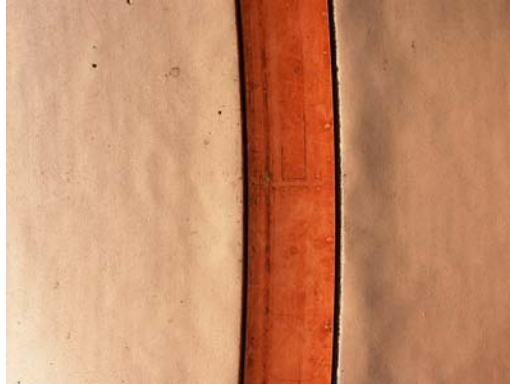
Figure 66. Features on the Cu in the vicinity of a radial groove on the vacuum chuck. The photograph is representative of most of the features on the Cu.
