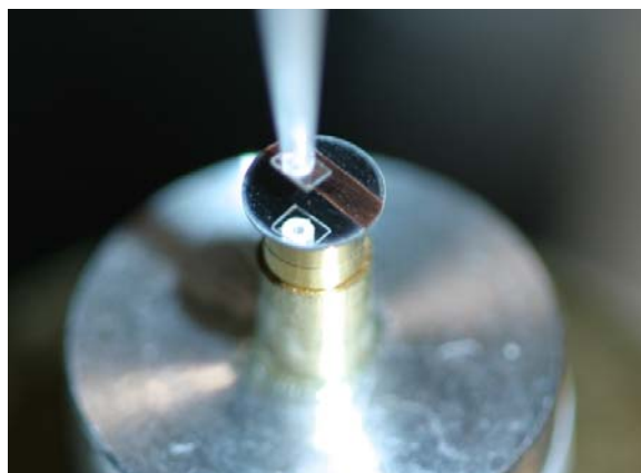
Figure 73. Alignment of a quartz window on an EOS target
