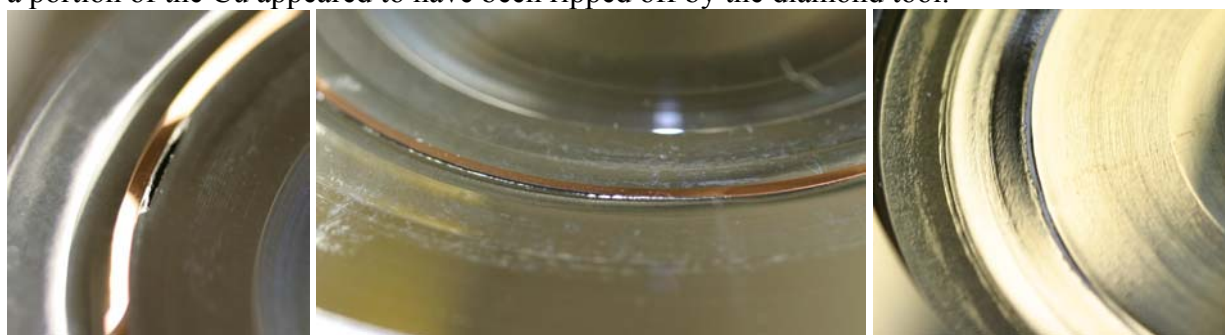
Figure 47. Disk D2 after being machined to a thickness of 90 \mu\text{m} . Small rip on inside of Cu (left), large clean cut through outside of Cu (center), large rough cut 1 mm inside the Cu on the machined face of the Al (right)
