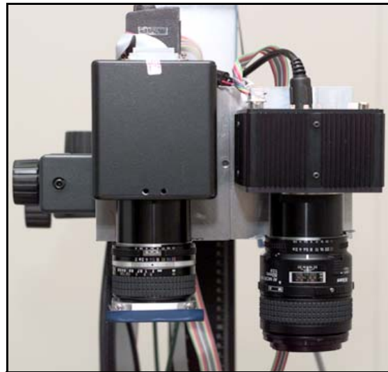
Figure 5: Initial dual-band benchtop prototype camera system for measuring moisture content consisted of a CCD linescan camera (left) for measuring light scattering in the visible range, and an InGaAs near-infrared linescan camera (right) for measuring water absorption at 1.45\mu .
