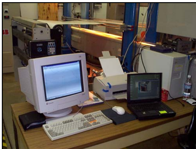
Figure 8: A new PC-based data acquisition and processing system was developed to replace the bulky VME based system used in the past.
