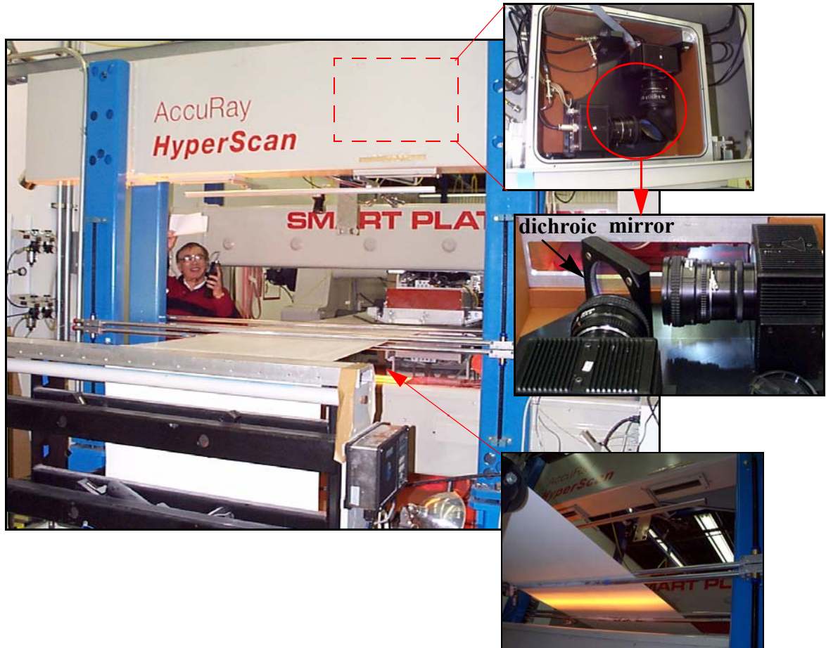
Figure 9: Improved camera system is repackaged to fit inside ABB’s HyperScan system and uses a dichroic mirror for providing a single optical axis to reduce camera alignment errors.
