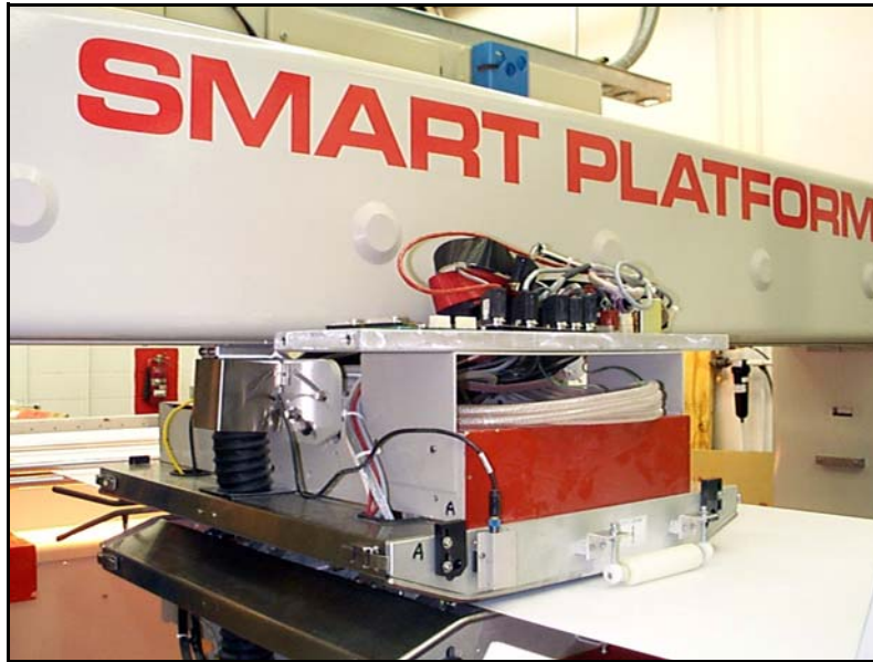
Figure 1: Commercial scanning system for measuring paper properties during production.
