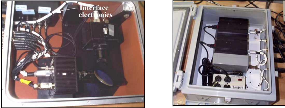
Figure 14: Camera interface electronics was modified and repackaged to fit inside the Hyper-Scanner case, power supplies are repackaged in a ruggedized and watertight case.
