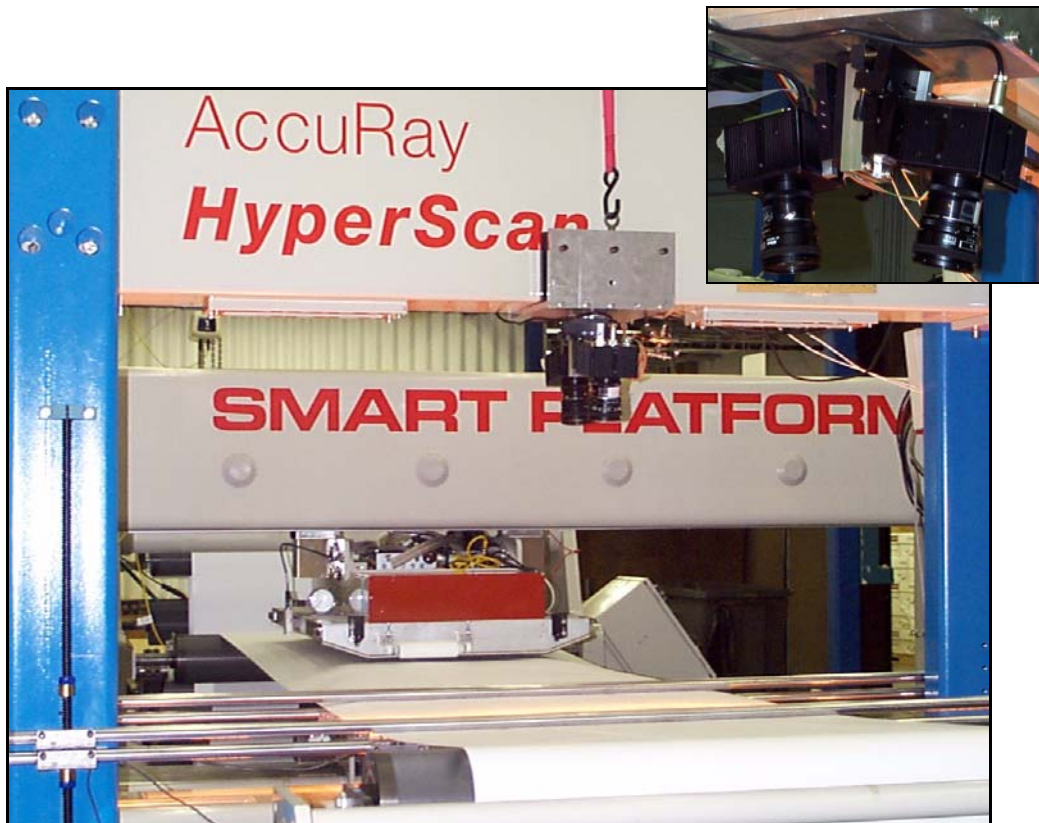
Figure 6: A proof-of-principle prototype linescan camera system for continuously measuring moisture content on moving paper was installed and tested at the Matilda testbed. The system made use of two InGaAs linescan cameras to measure transmitted light at 1.45\mu and 1.1\mu .
