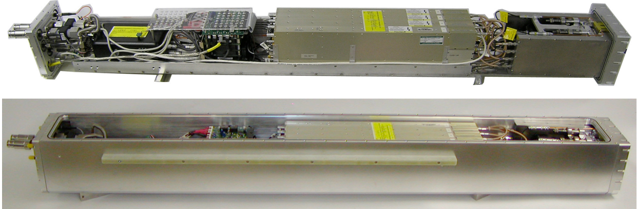
FIG. 1. The Gated X-ray Detector pulled outside of the air box (top) and within (bottom). Various types of imaging and spectrometer nosecones can be placed in front of the detector when the instrument is in the NIF vacuum chamber.
