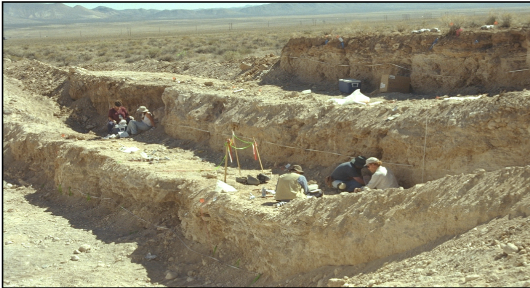
Figure 12. Photograph of vadose zone trench at the NTS from which samples were collected for ^{129}\text{I}/^{127}\text{I} and ^{36}\text{Cl}/\text{Cl} analyses.
