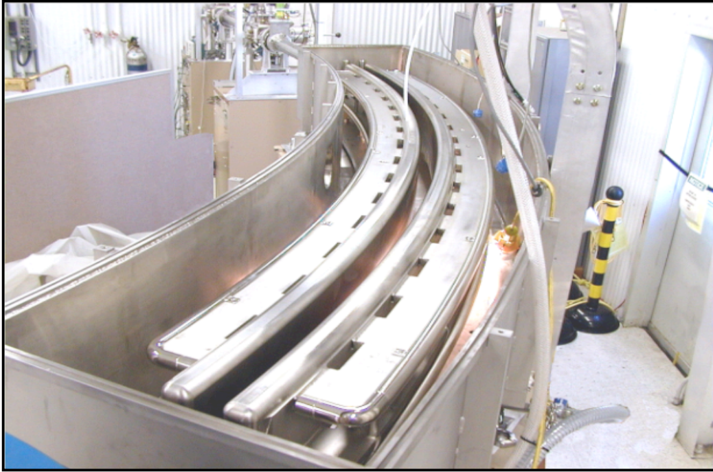
Figure 3. Close up of the high energy electrostatic analyzer without top cover plate. Note door to right for scale. The two curved plated to each side of the center beamline carry the positive and negative charge that deflects the ion beam and creates an energy spectra further isolating ^{129}\text{I} .
