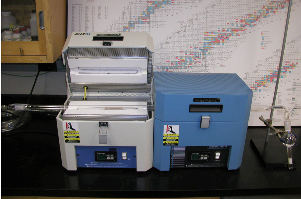
Figure 14. Photograph of the double furnace array used for combustion of soils to extract iodine. Sample placement can be seen within the glass tube in open furnace to left. Oxygen is passed through the tube from the left and the iodine is trapped in the solution in the flask to the right.
