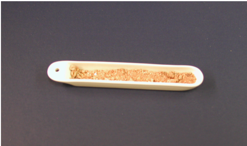
Figure 15. Ceramic boat used to hold soil sample in combustion furnace. Expanded soil sample can be seen in the boat. The boat is approximately 3 inches long.
