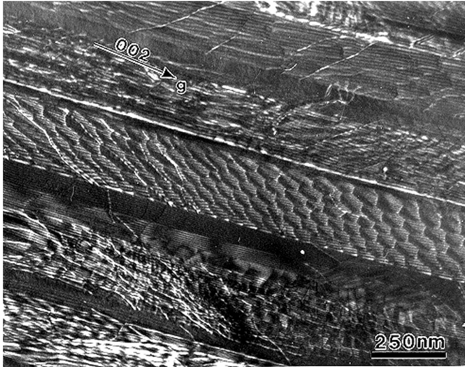
Fig. 13. A weak-beam dark-field TEM image showing the zigzag motion of interfacial dislocation array observed within a specimen creep deformed in the LS regime ( 760^{\circ}\text{C} , 136 MPa).
