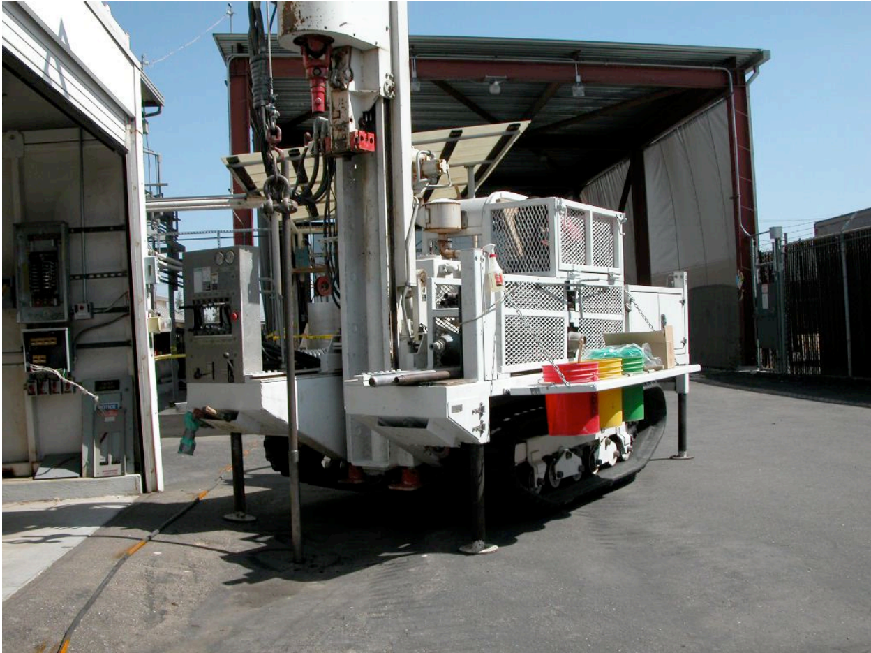
Figure 4-2. Direct Push Sampling Rig
