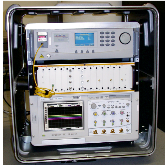
Figure 4. The 4-channel heterodyne system is packaged into a portable case. From top to bottom are the 2-W fiber laser, the custom fiber/detector chassis, and the high bandwidth digitizer. The digitizer shown here is built by Agilent Technologies; it has 6-GHz bandwidth and a sample rate of 20 GS/s on all four channels simultaneously for 50 \mu s.
