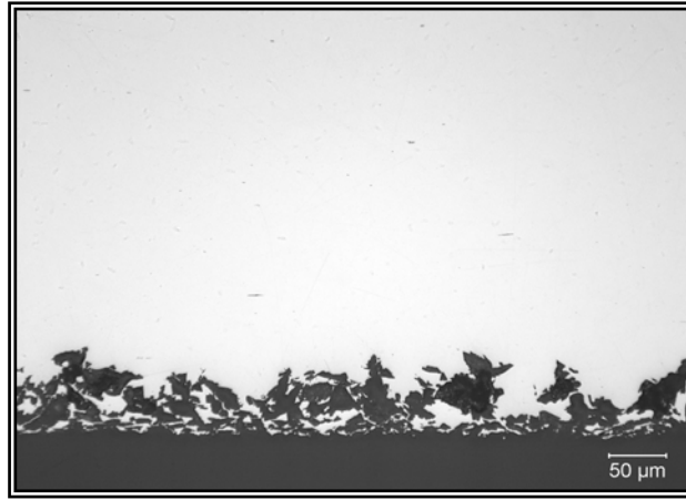
FIGURE 5 - Internal Attack of Non-Stressed Annealed C-22HS Alloy in 20% HF at 79°C (Medium Magnification-Unetched)
