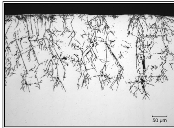
FIGURE 9 - Internal Features of Stressed N06022 in 20% HF at 79°C (Medium Magnification-Unetched)
