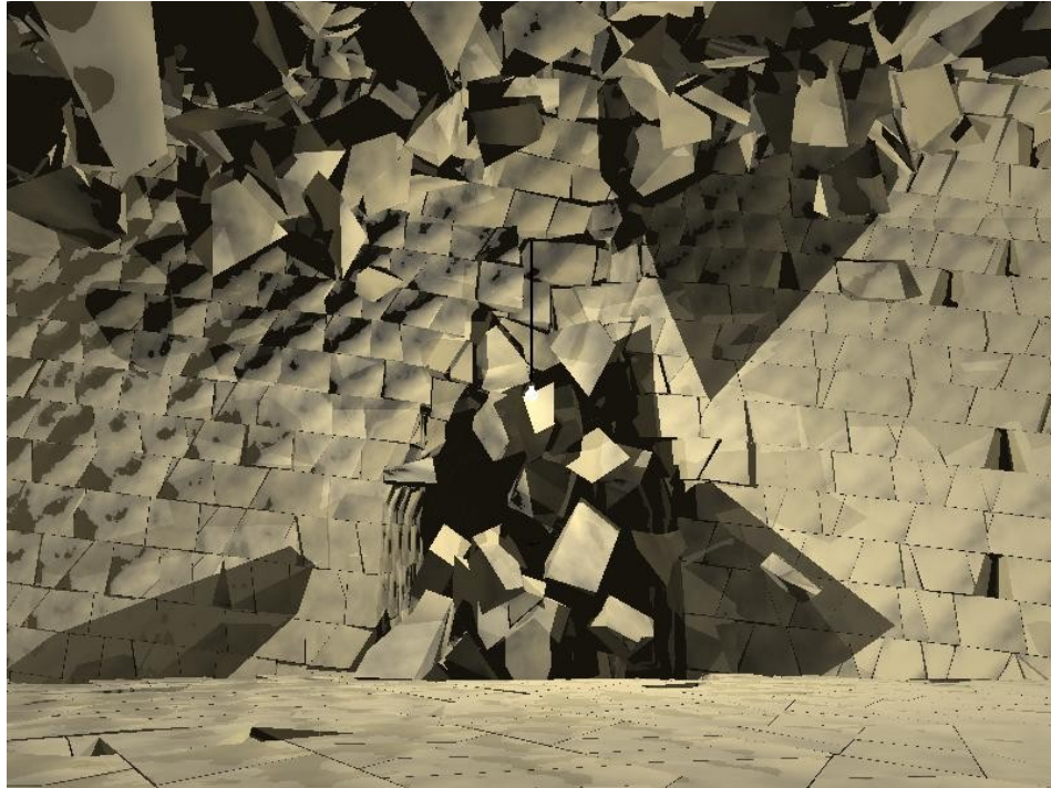
a) The small tunnel seen from the upper chamber at 300ms appears to be completely destroyed
