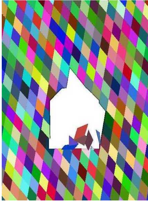
LDEC simulation showing a non-symmetrical roof failure controlled by jointing
