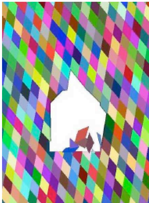
b) LDEC showing a non-symmetric roof failure controlled by the jointing
