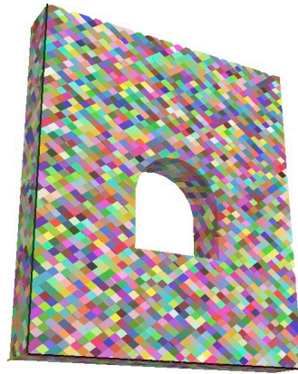
a) Rock island, with 3 joint sets and 12425 blocks, loaded on the top with a velocity pulse
