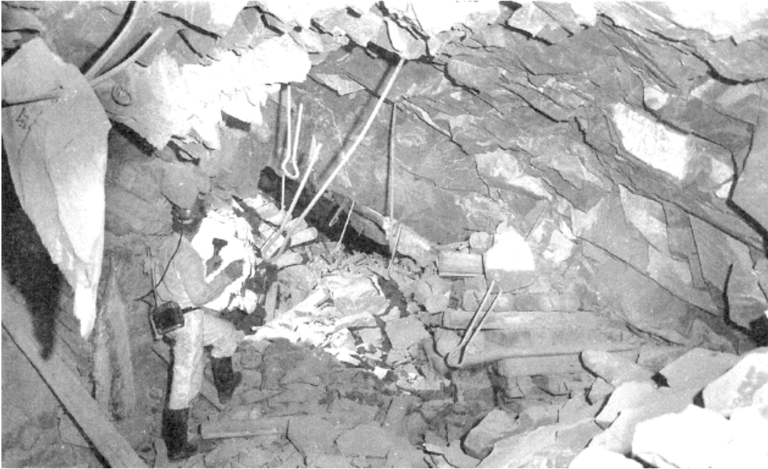
a) Fairly symmetrical roof collapse and floor rubble due to a rock burst in a South Africa gold mine (courtesy of Dr. Ortlepp, 2003)
