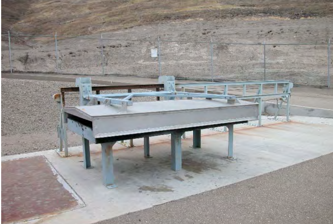
Figure 3. EWTF burn pan, covered. (UCRL-Photo-213179, July 16, 2005)
