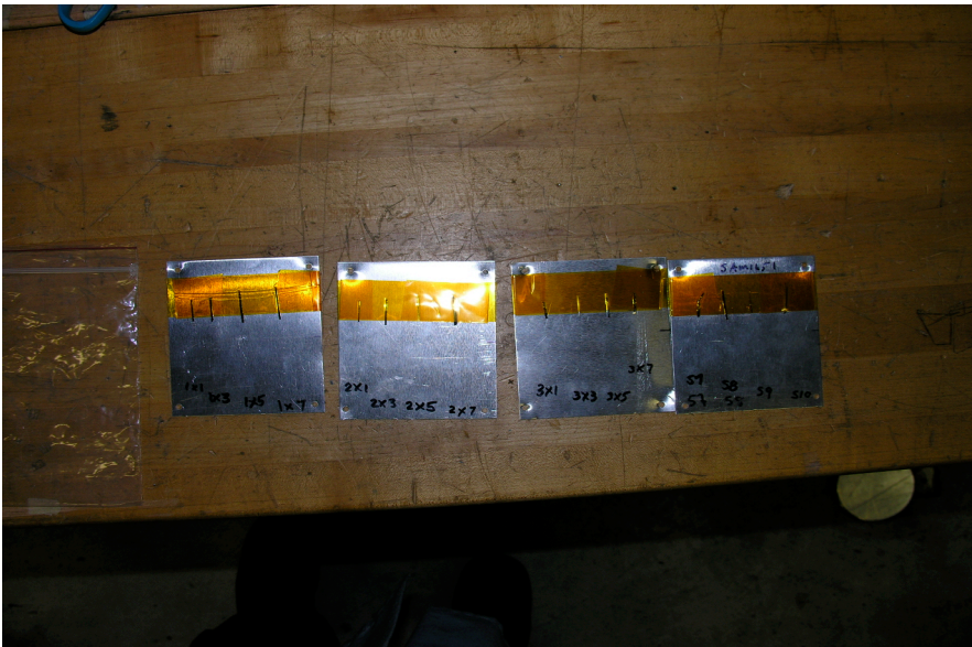
Figure 10 Four Series of Melt-Spun Ribbons Taped on Aluminum Plates
