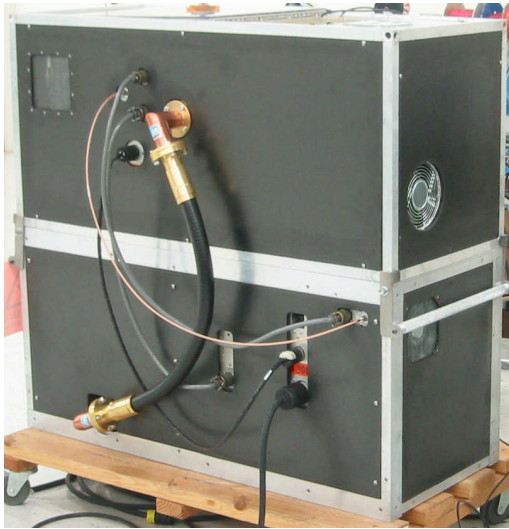
Figure 7 Photograph of fully assembled portable RFQ 60 keV neutron generator
