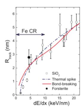
**Fig. 5:** Amorphous track radius vs. electronic stopping power dE/dx. Experimental data points are for forsterite (this work) and quartz (Meftah A. et al. 1994). The lines are results of the thermal spike (Szenes 1997) and bond-breaking (Tombrello 1994) model predictions. The dE/dx range for 0.1-10 GeV Fe cosmic rays in forsterite is also shown.
