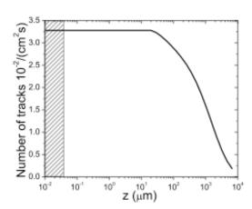
**Fig. 6:** Track density for Fe CRs with energies larger than 100 MeV as function of depth. The dashed box indicates the range of typical Fe solar wind ions with ~1 keV/amu. Solar flares with higher energy ions would penetrate deeper.
