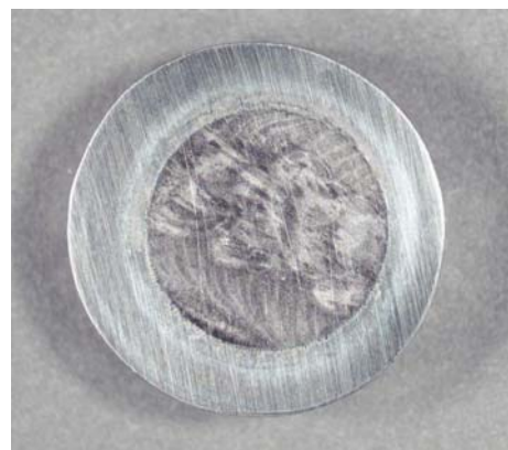
Figure 18. Specimen G03A (GTAW) after galvanostatic treatment of 1 mA/cm 2 for 3 h in 1 M HCl at 60°C
