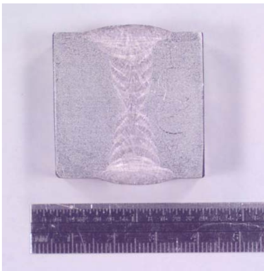
Figure 1. Macrograph of a GTAW welded Alloy 22 plate
