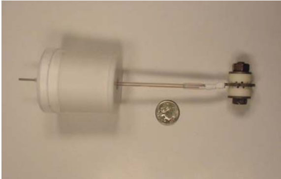
Figure 3. MCA Specimen for Crevice Corrosion Testing
