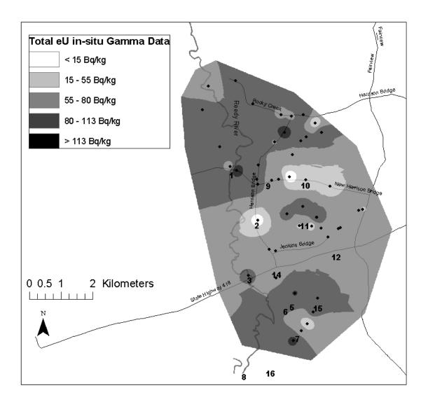
Figure 1: Contour maps developed using eU concentration obtained from *in-situ* gammaray spectroscopy. The numbers represent the location of the river and stream sampling while the diamonds represent the location of the *in-situ* measurement. Sampling area is in the vicinity of N 24° 39.0' and W 82° 16.5'.
