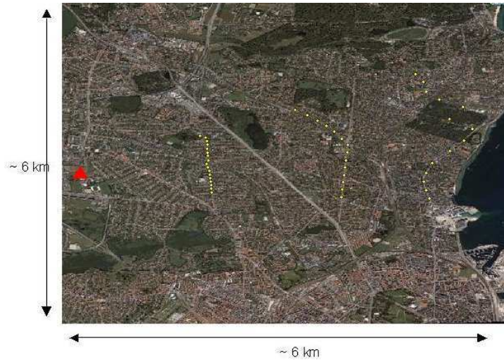
Figure 10: Domain of the Copenhagen experiment. The red triangle denotes the actual source location and the yellow dots indicate the three arcs of SF_6 sensor locations. The most distant sensors are approximately 6km from the source.
