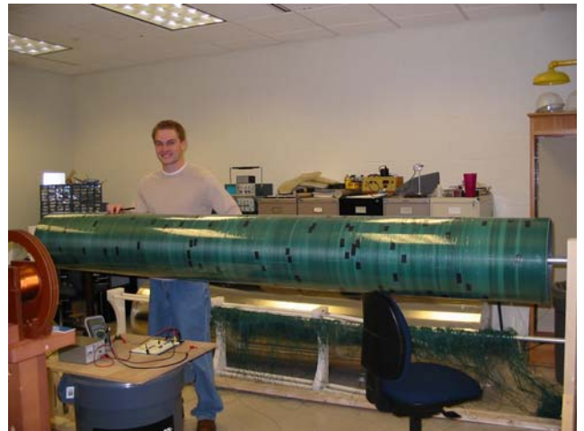
Figure 2: Extremely uniform static magnetic field with a magnetic field of 1.78Gauss.
