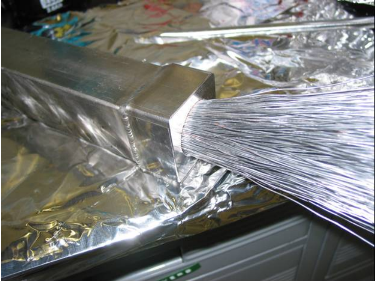
Fig. 6. Transition piece welded to the CS2 conductor.
