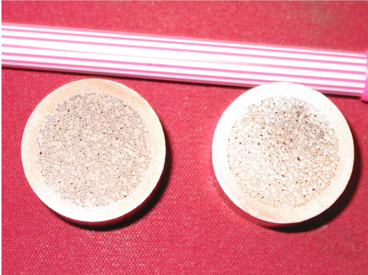
Fig. 11. Compacted and sliced cables in the copper sleeve.
