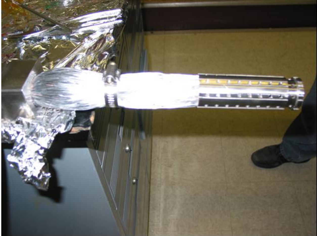
Fig. 9. The flow distributor is stuck on the cable and would not go.
