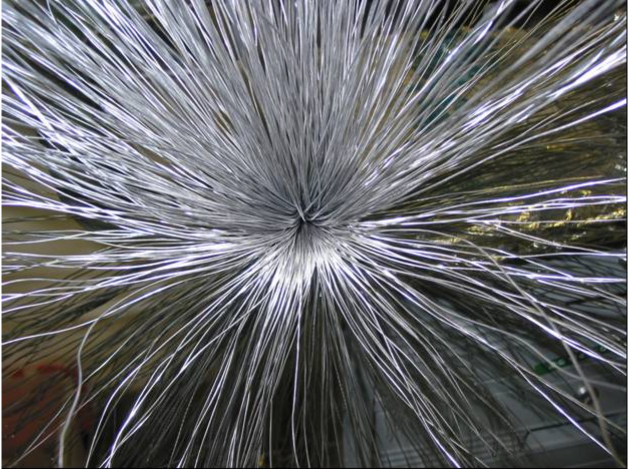
Fig. 7. Cable with the spread strands.
