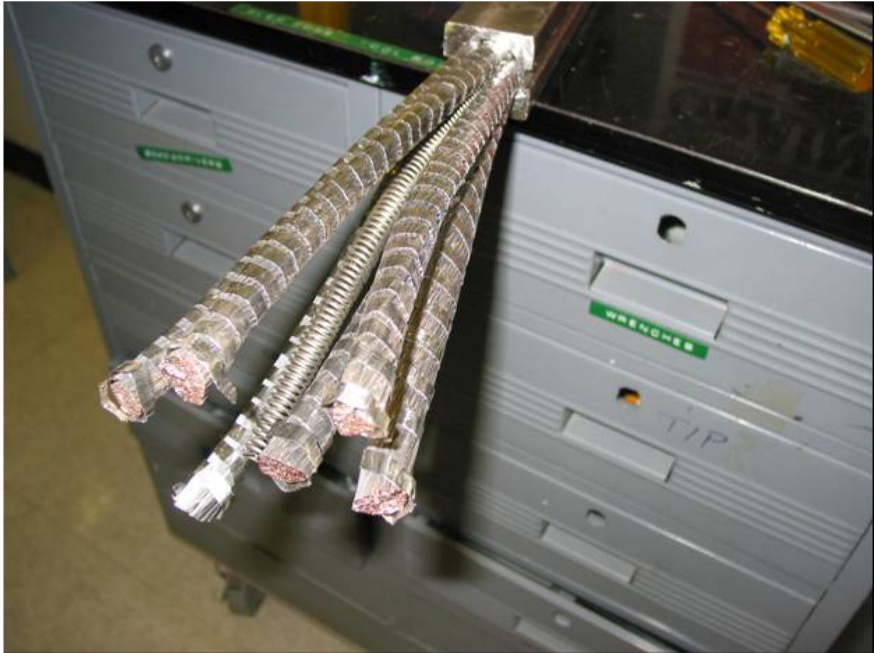
Fig. 4. The CS2 CICC after the jacket is stripped off and the outer wrapped is removed.
