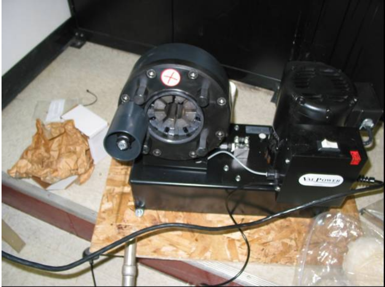
Fig. 10. Hydraulic crimper used for compacting the cable in the copper sleeve.
