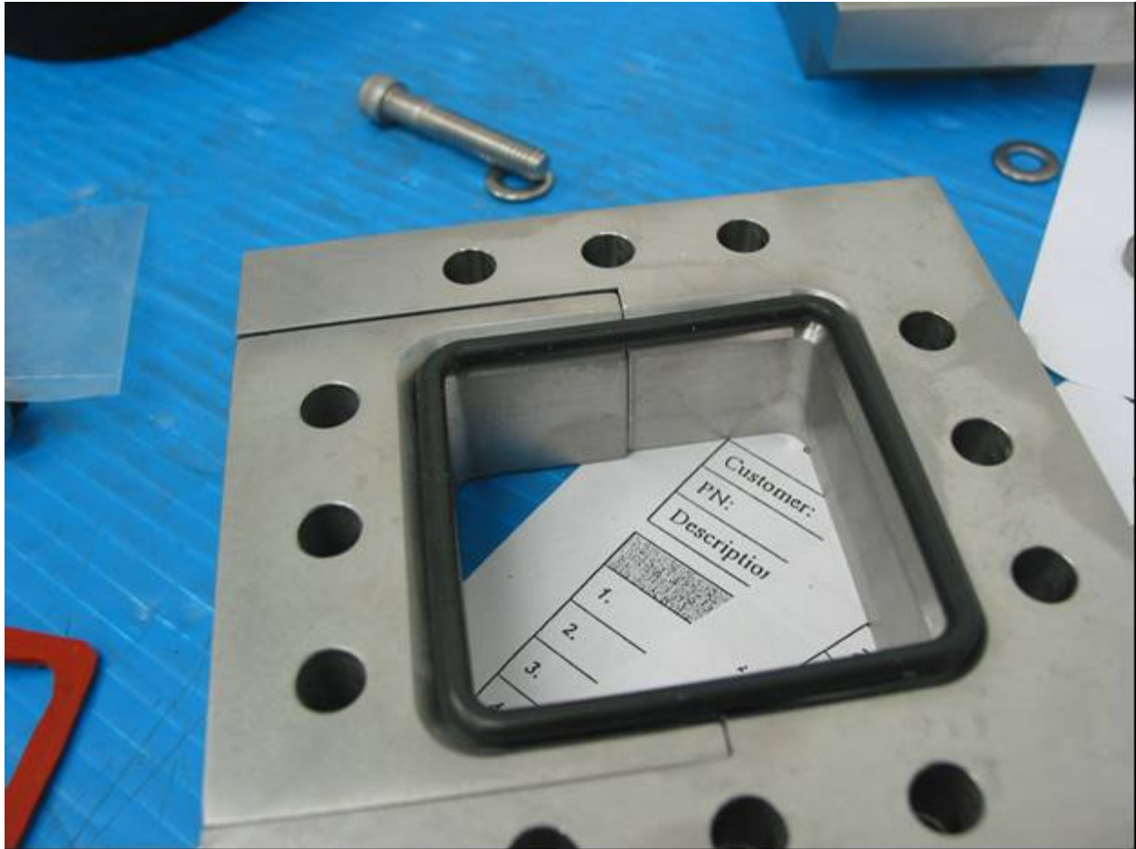
Fig. 14. The O-ring cross section is too small to seal around conductor.
