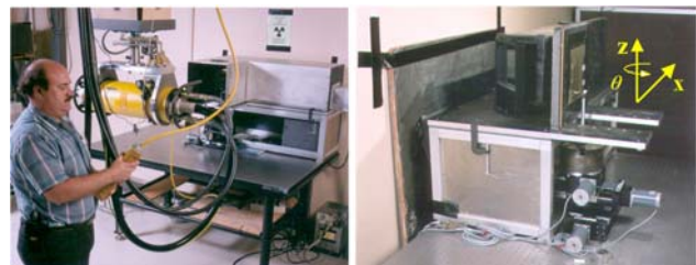
Figure 6: Photograph of the PCAT digital radiography and computed tomography system (left). Photograph of the inside of the PCAT detector box (right).
