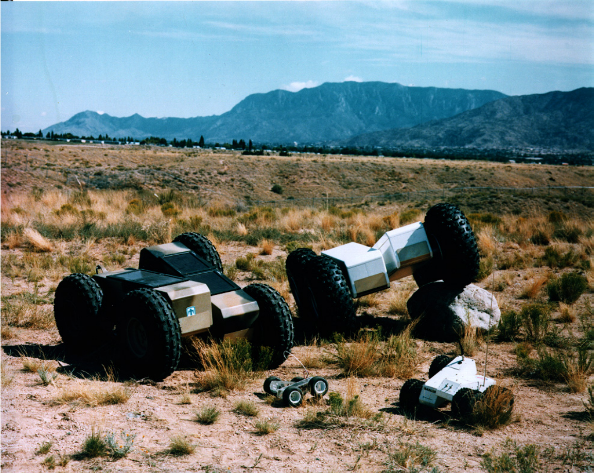
Figure 2 – The RATLER™ Robotic Vehicle Family
