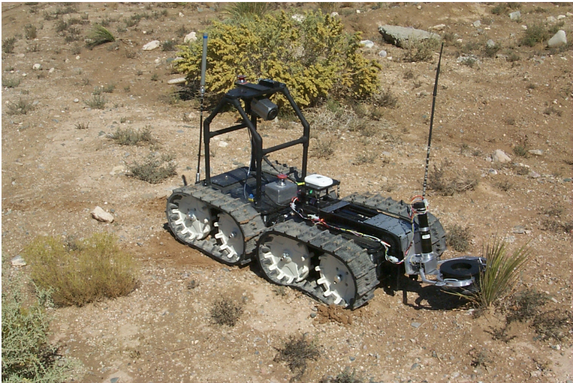
Figure 47 - SandDragon Vehicle Holding Sensor Pod Replica
