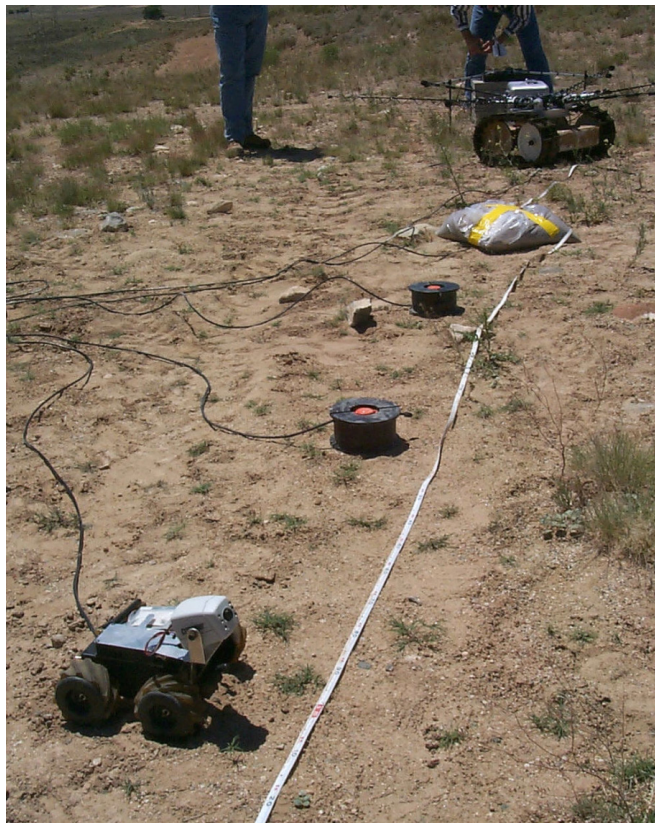
Figure 4 – Seismic Coupling Test Layout
