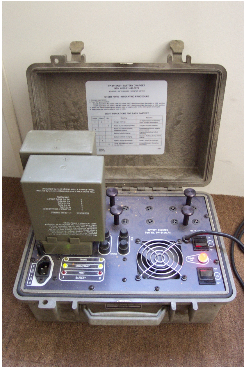
Figure 20 - Charger for Li-Ion Rechargeable BB-2590 Battery
