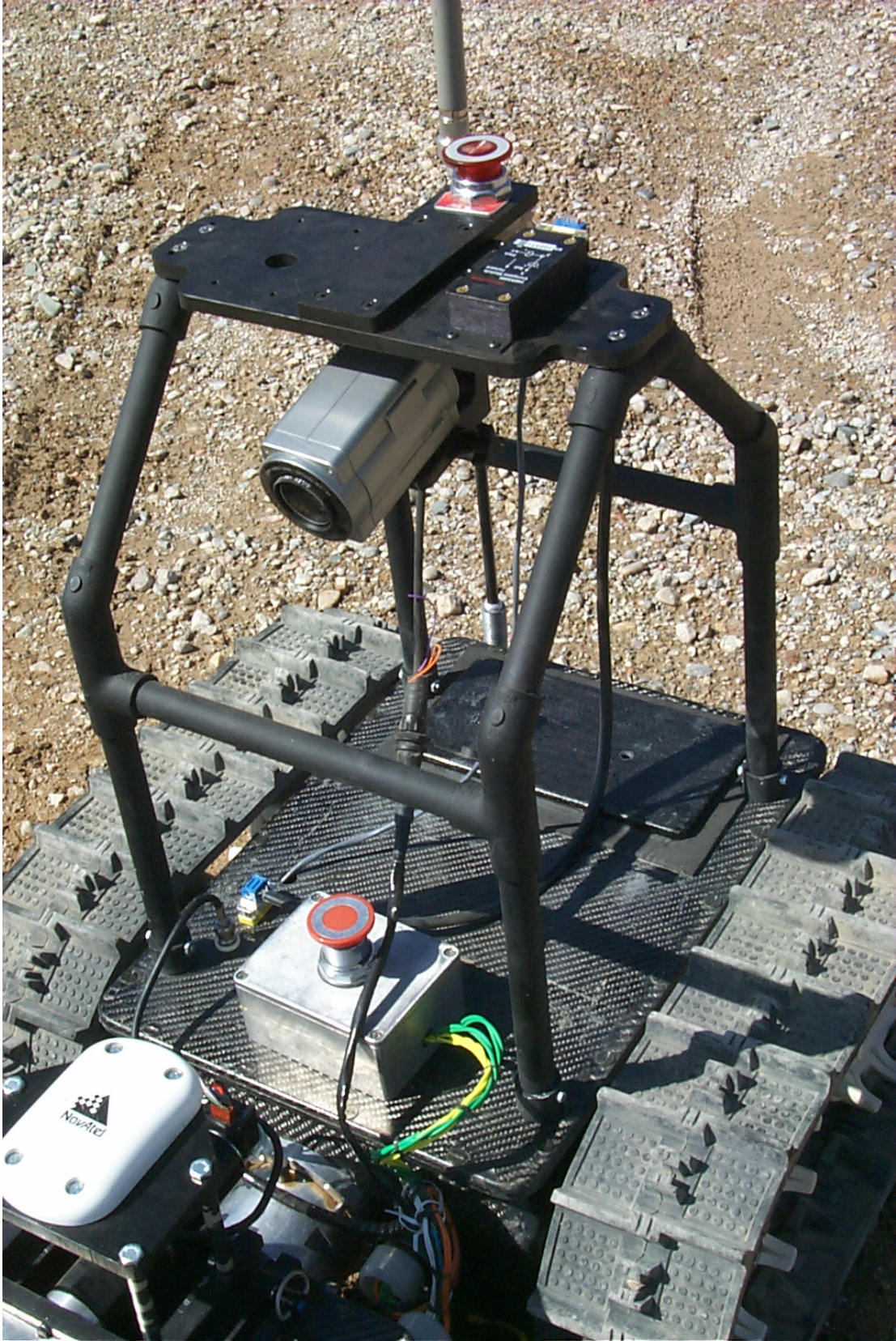
Figure 26 – SandDragon Robotic Vehicle Rear Body Sensor Support Structure
