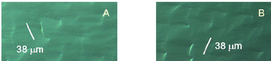
Fig. 10. Nomarsky optical images of 10a) 15.0% In 5 MQW, and 10b) 18.4% In 5 MQW surfaces showing presence of large ridge-like structures.
