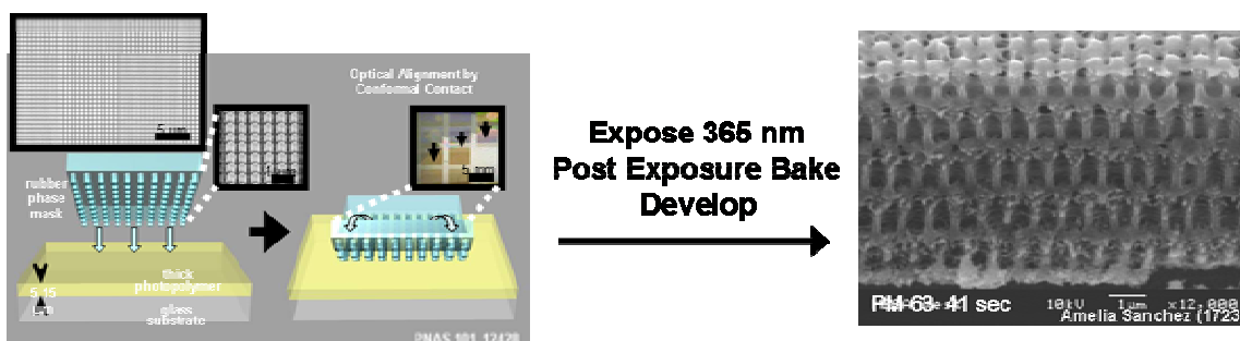
Fig. 17. Schematic cartoon of 3D structure fabrication with phase mask lithography and resultant 3D structure.
