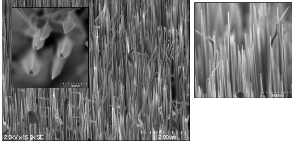
Figure 4. SEM images of highly aligned growth of GaN nanowires at 800 °C on r -plane (1-102) sapphire
