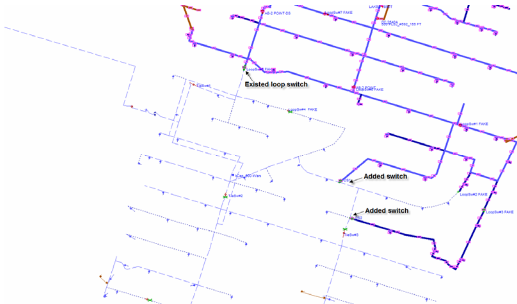
FIGURE 17 Location of opened switches of reconfiguration without DG at August, Tuesday 3 AM
