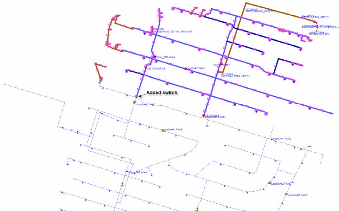
FIGURE 14 Location of opened switches of reconfiguration with DG at August, Tuesday 3AM
