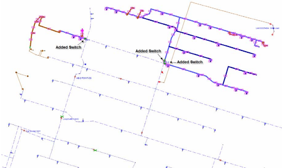
FIGURE 11 Location of opened switches of reconfiguration with DG at minimum load time point
