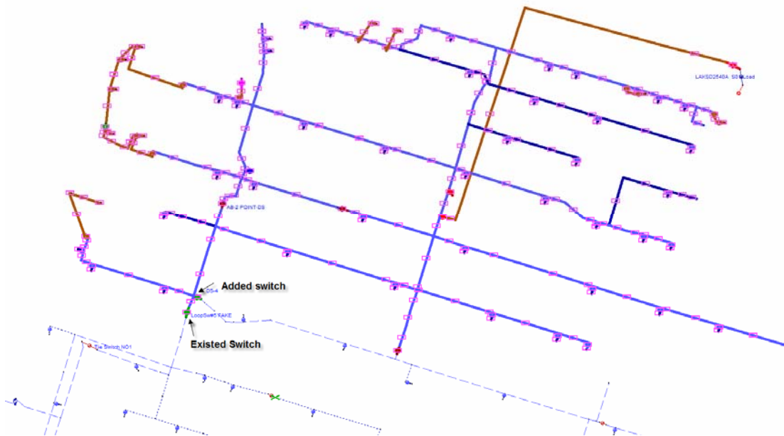
FIGURE 12 Location of opened switches of reconfiguration without DG at minimum load time point
