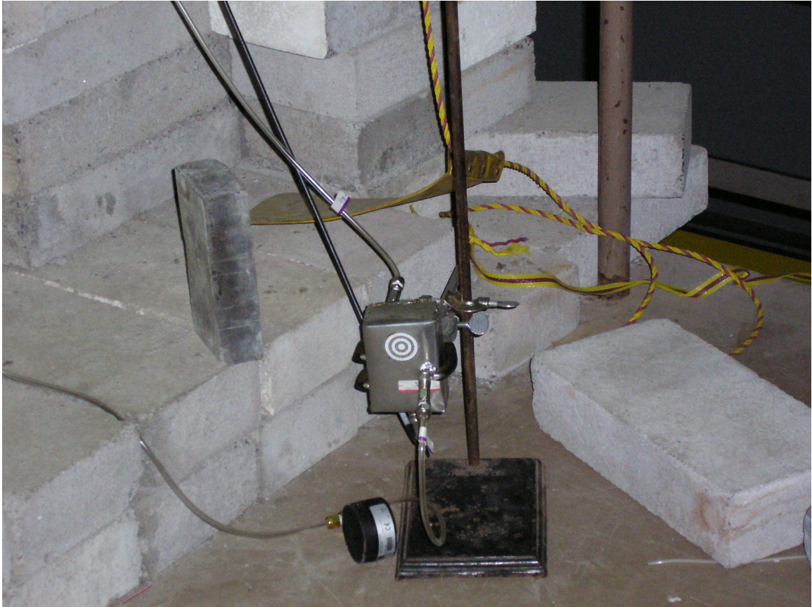
Figure 5.5. GEM-base TEPC in the radiation area.
