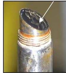
Silicon adhesive covering Sol-gel
