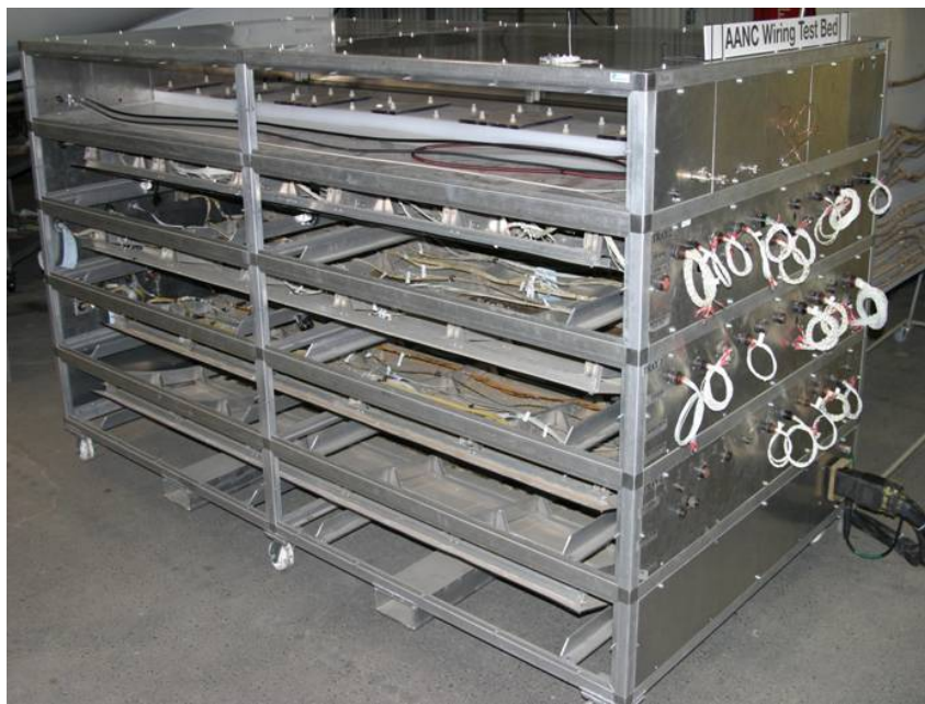
Figure 28: AANC Wiring Test Bed
