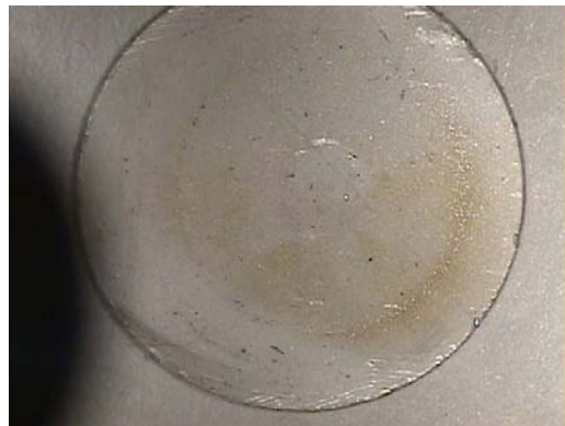
Figure 17: Microscopic photograph of mylar sample after high energy pulse.
