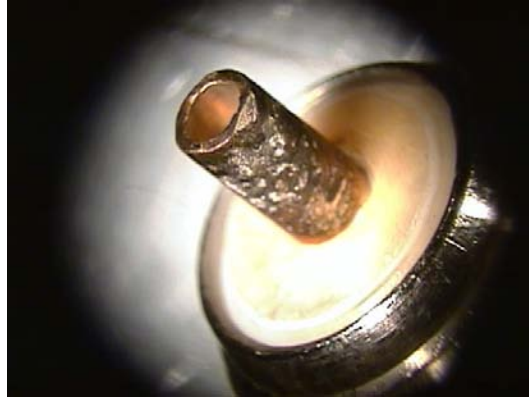
Figure 18: High voltage electrode following insulation material testing.
