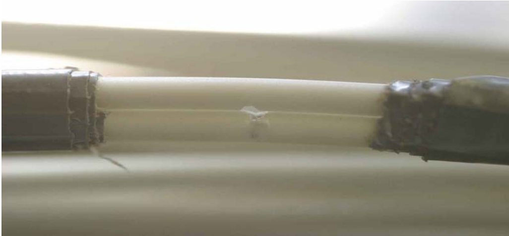
Figure 24: Wire to wire defect
