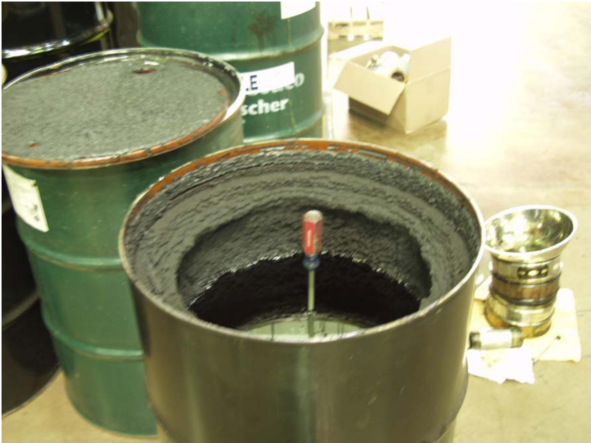
Figure 4-4. Drum of RCO Bottoms prior to heating.
