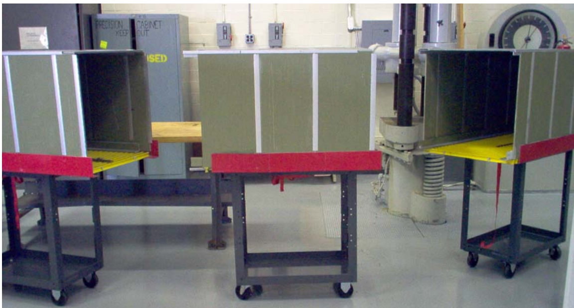
Figure 4.9 Unassembled Sections of the Model Trailer
