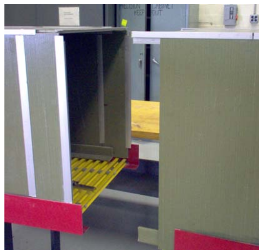
Figure 4.11 A Method to Assist the Joining of Segments for the Modular Application of the Van Trailer Design
