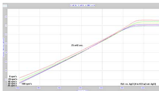
Fig. 2.1: Mass transport of Sb and Bi in DMSO at low convective agitation.
