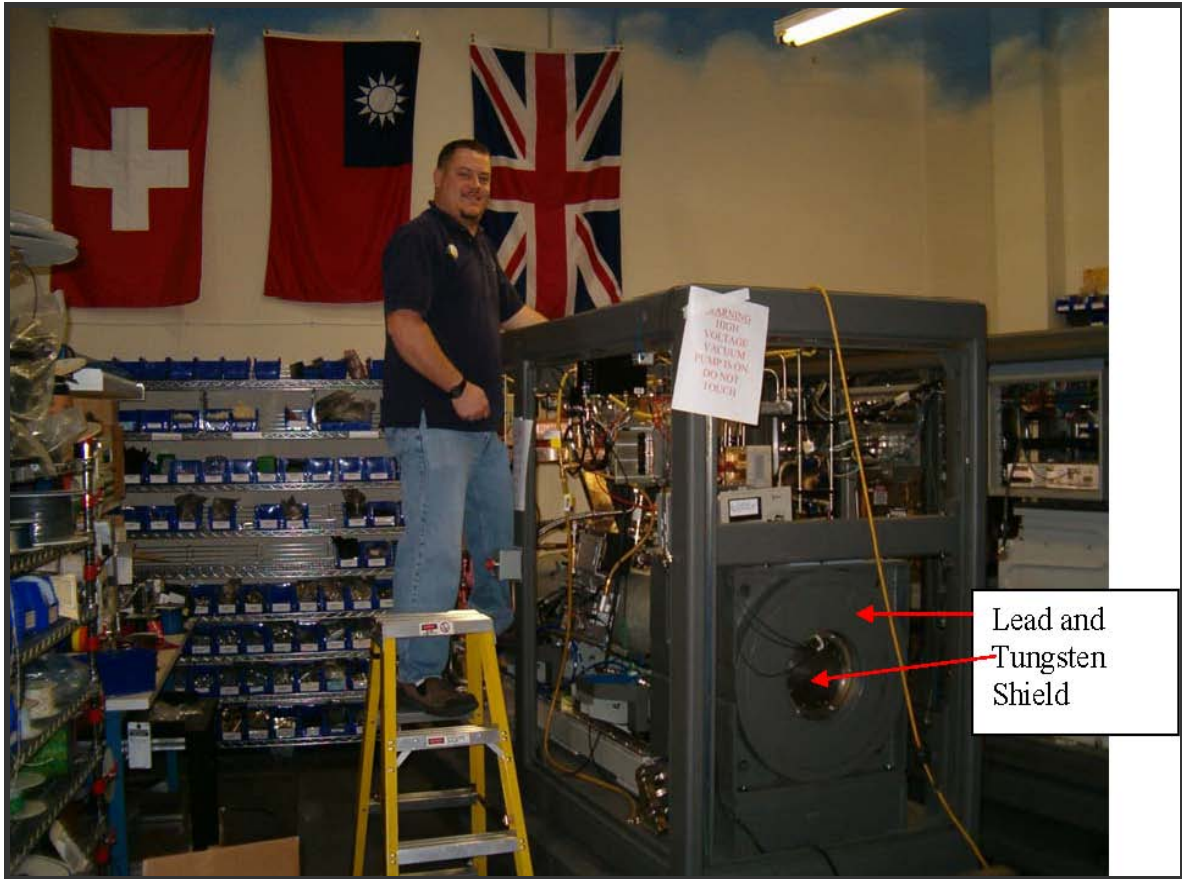
Front view of the K9 system X-ray head front view truncated from the RF unit. The klystron, klystron pulse tank and solenoid are shown rear view of the accelerator, showing the triode electron gun and the dual energy triode gun pulsar system front view of the modulator cabinet. Power distribution, the solenoid magnet power supplies for the klystron and accelerator are in this cabinet. One PLC rack is also in this cabinet.
