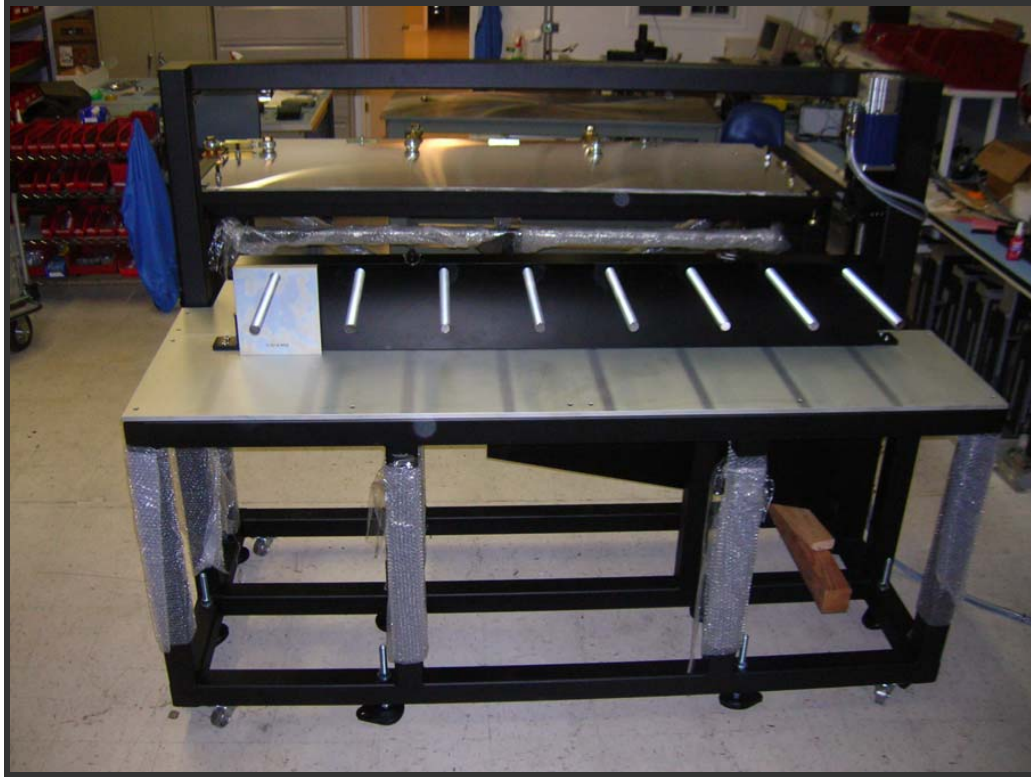
Front view of sample table. 14" steel or other material can be stacked in front of the detector array. The steel has already been ordered and delivered as part of this program.
