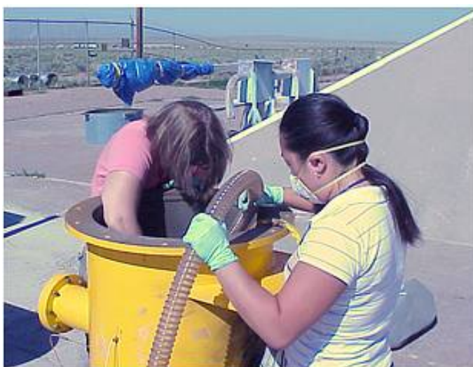
Figure 6.13 HEPA Vacuum Sampling of Post-test Aerosol Chamber Particulate Debris
