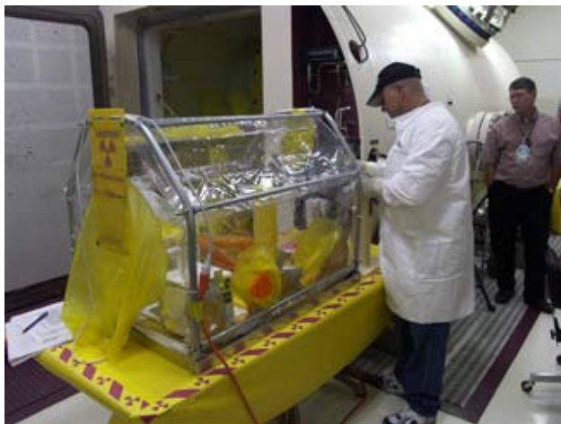
Figure 6.20 External Glove Box for Aerosol Sampling
