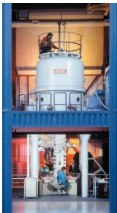
The National Center for Electron Microscopy, Lawrence Berkeley National Laboratory. Its newest microscope can resolve atoms that are less than 0.1nm apart.
