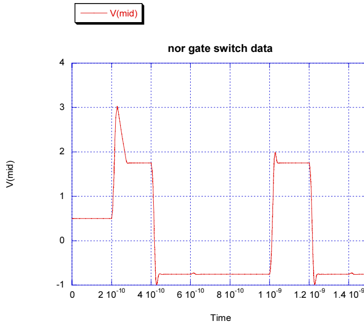
Figure 25: NOR gate switching with .06 W pulses.
